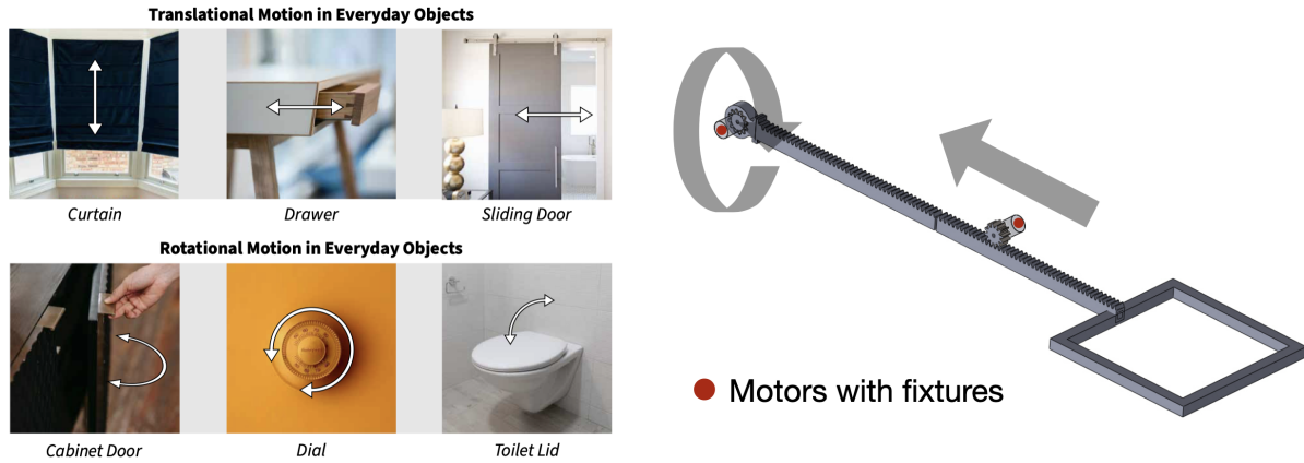
Fig. 1. Translational and rotational motions are the two common types of motion on everyday objects (left). The device designed to simulate these motions on everyday objects and used in the energy investigation tests (right).
