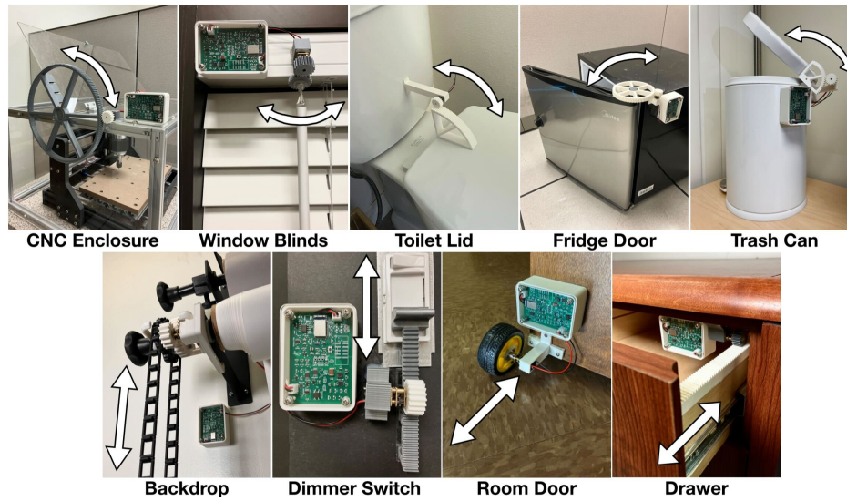
Fig. 7. MiniKers instrumented on 9 everyday objects, enabling self-sustaining automatic operations. Top row shows objects with rotational movements and bottom row with translational movements.
