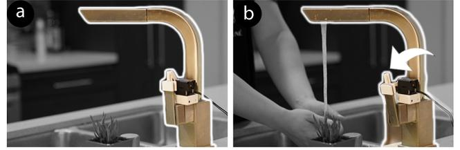
Figure 6. A manual faucet can automatically turn to release water by attaching a mechanism to pull the handle.
