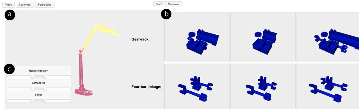
Figure 3. A screenshot of the user interface provided to the user once Robiot generated a set of candidate mechanisms from a given video demonstration: the corresponding 3D model (a), the generated mechanisms (b), and sliders to filter the list by range of motion, torque and speed (c).
