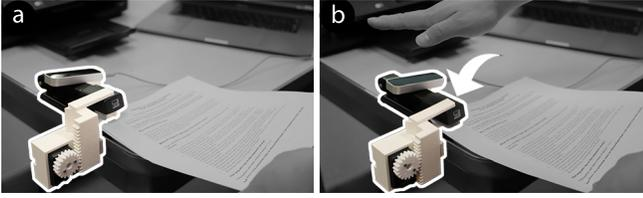
Figure 4. Automatic stapler is one common office appliance, that Robiot can robotize from a cheap manual stapler
