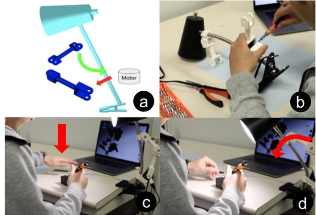
Figure 14. Robiot generates an instruction for assembly (a), then a participant can assemble and install following that instruction (b), to interact with the robotic things using gesture (c) lowering the lamp height to work with optimal brightness when soldering (d)
