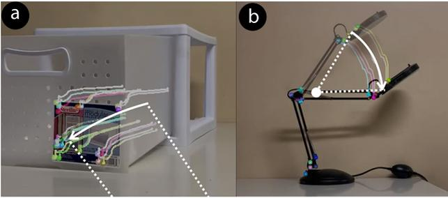
Figure 8. Optical flow analysis shows distinct difference between prismatic (a) and revolute (b) joints by comparing the least-square fitted radius (prismatic joint’s fitted radius is much larger, extending beyond the camera view).
