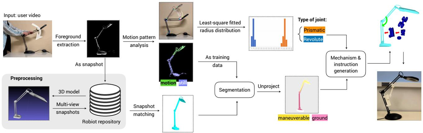
Figure 2. Overview of Robiot's end-to-end pipeline for generating actuation mechanisms from a user's input video.
