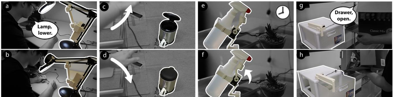
Figure 1. Robiot enables end-users to take a video and automatically generates mechanisms that can actuate everyday objects to perform simple physical tasks. All the four examples were designed by participants in our design session: lowering a lamp while busy soldering (a), waving a hand up to open a trashcan afar (c), setting up a scheduled house plant water spraying system (e), and asking the drawer to open itself when having no extra hand (g).
