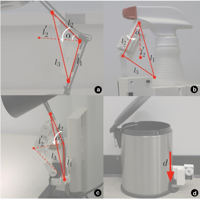
**Figure 11.** Three mechanisms and their parameters (gear rack appears twice for both types of joints). For revolute joints, different mechanisms can be considered and modeled after the same set of parameters –  $l_1, l_2, l_3$  and  $\alpha$ .
