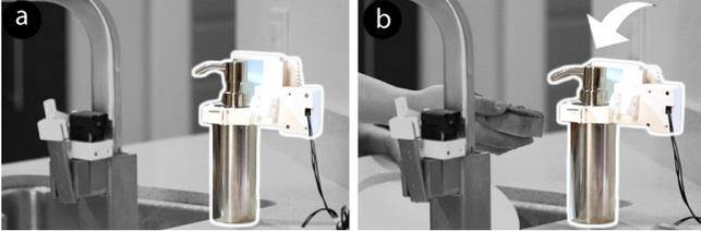
Figure 5. Robiot mechanism attached on top of a soap bottle performs pressing to squeeze liquids without touching
