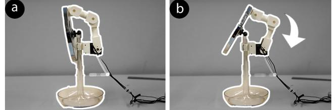
Figure 7. Automatically adjusting mirror can aid a user who wears make-ups and contact lens using both hands
