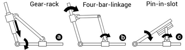
Figure 10. Technical sketches of the three mechanisms showing how they are actuated.
