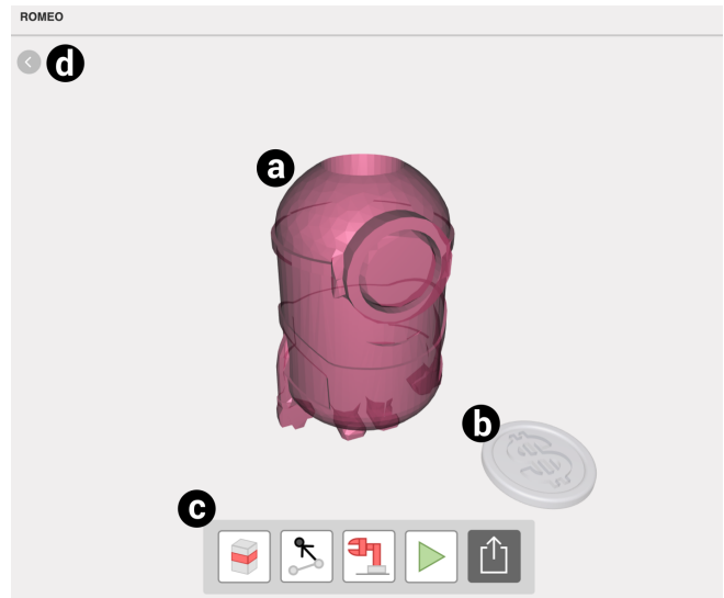
Figure 3. A screenshot of Romeo’s user interface: a) target object; b) reference object; c) functional buttons, from left to right: selecting transformable part, specifying motion points and action, generate embedded robotic arm, animation, export and d) button to restart the current step
